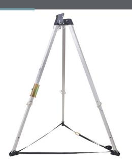
This Confined Space Tripod is essential when working in a confined space to ensure safety requirements are met. This tripod has adjustable sliding telescopic legs with a load capacity of 500 kg.
